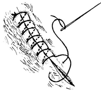
Figure 3–10. Locking over-and-over stitch.
